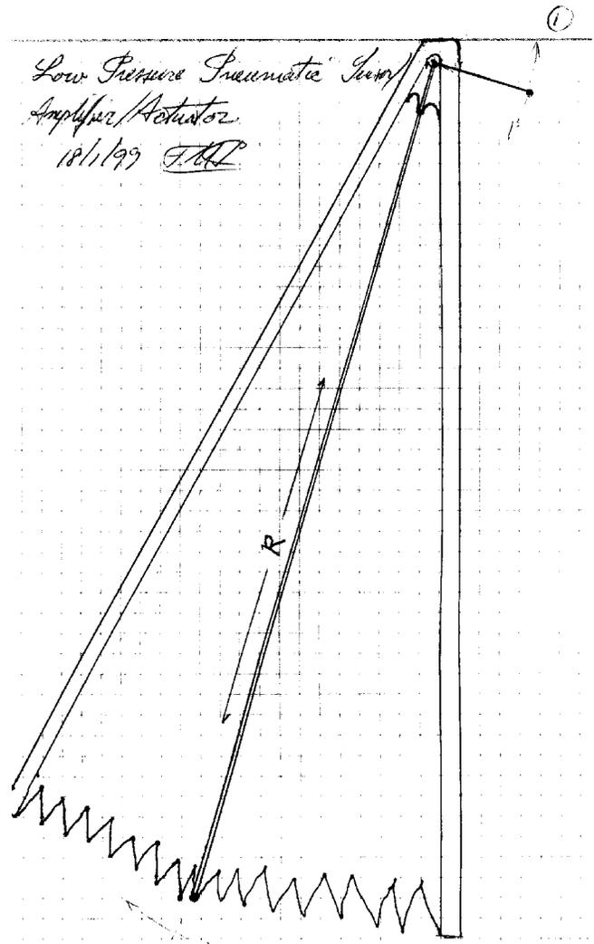
in such a way as to correct the deviation, in accordance with the well-known principle of closed-loop or feedback control. Because this effect is proportional only (no integral effect), the error is not brought to zero except at one ("design" or "ideal") power setting, but skirt flow in confined to a narrower band than when a fixed splitter is used.
