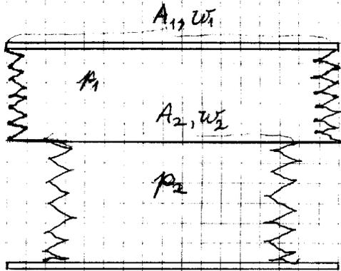
In the preferred embodiment, the actuator is fed from the plenum chamber directly into chamber  $A_1$  (the larger one), preferably through holes in a common partition rather than through external plumbing. The movable plate is
